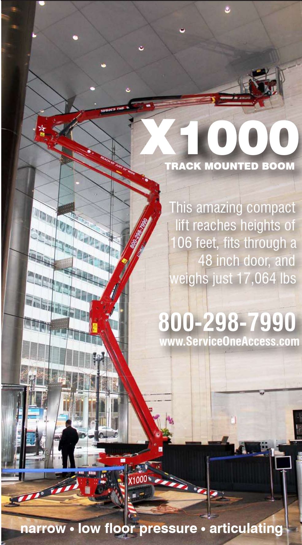
"Crawler" Drive Navigates Rough Terrain
